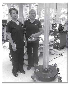
The Germaway UV-C light applicator is deployed in clinic pods (right), the back of the ambulances, and small rooms throughout the facilities. The goal is to destroy harmful microorganisms that might remain on surfaces after routine room and facility sanitizing.
